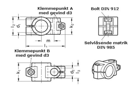
Adjustable clamp lever for d3 = GN 911-M 8-32 have to be ordred separately |1 = 81.5Adjustable clamp lever for d4 = GN 911-M 6-25 have to be ordred separately
